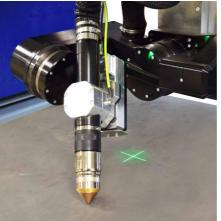
Laser for set up of program starting Triple torch unit point, optional with camera system
