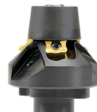
fig. 45°-radius-milling head with 3 x 2 cutting edges and guide roller, equipped with 3 x 3 mm-radius-indexable inserts of type R-K
