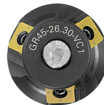
fig. 45°-bevel-milling head with 3 cutting edges and guide roller, equipped with 3 bevel-indexable inserts of type K
