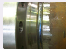
Tube-flange connection welded with manual SAW equipment
