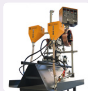
Modification for the welding of trapezoidal sheets
