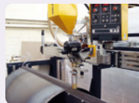
KA 2-UP for longitudinal welding with backing bar
