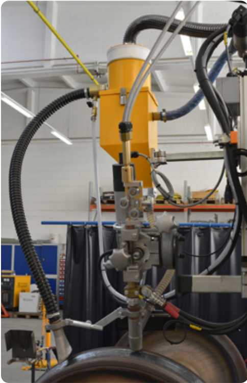
Flux container 10 l with pressure and suction hose
