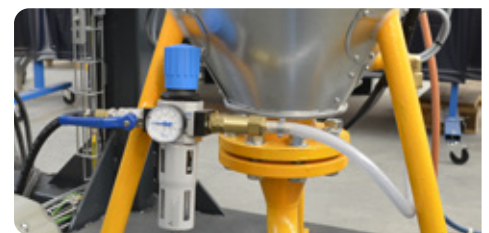
Pneumatic maintenance unit
